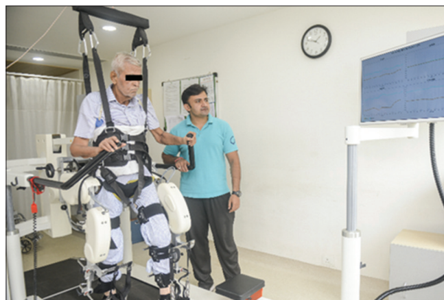
Figure 6: Lokomat: Robotic assisted gait trainer
